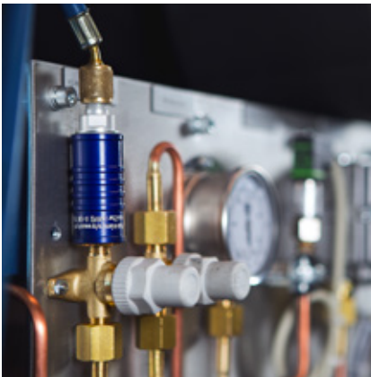
TW111 | For filling and evacuating of industrial refrigerating and air conditioning systems
