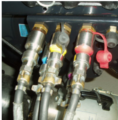
TW110 | For filling and evacuating of automotive air conditioning systems during production
