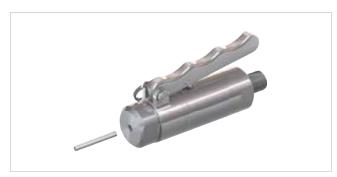
The WEH® TW141 Quick Connector provides pressure-tight connections on straight tubes and has earned a reputation for ease of operation. The TW141 is a lever-actuated connector, which creates no lateral forces that can distort the test piece or filling port when connecting and disconnecting. WEH® TW141 is fitted with an internal safety
