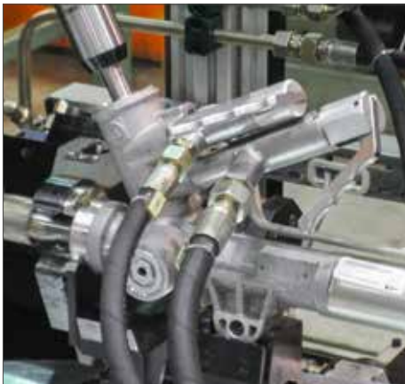
TW17H for testing of steering racks
