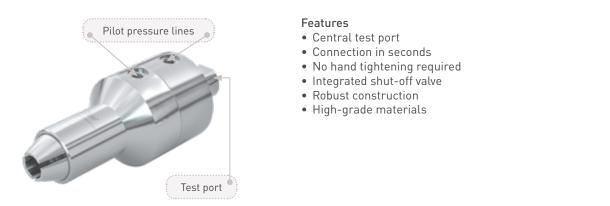
The WEH<sup>®</sup> Connector type TW713 has been specifically developed to connect fuel lines for engine hot testing and for testing of automotive components during manufacturing. The design of the connector is best suited for narrow spaces and meets the demand of such applications. Type TW713 is equipped with a central test port and pneumatically actuated grip sleeve for ease of use.
